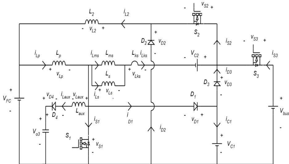
**Fig-6:** Bidirectional converter (Step down state)
