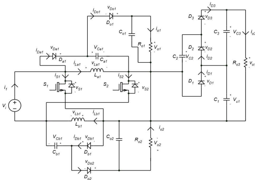
**Fig-11:** Single input three output non-isolated converter
