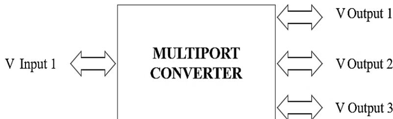
Fig-1: Basic block of multiport converter (SIMO Topology)
