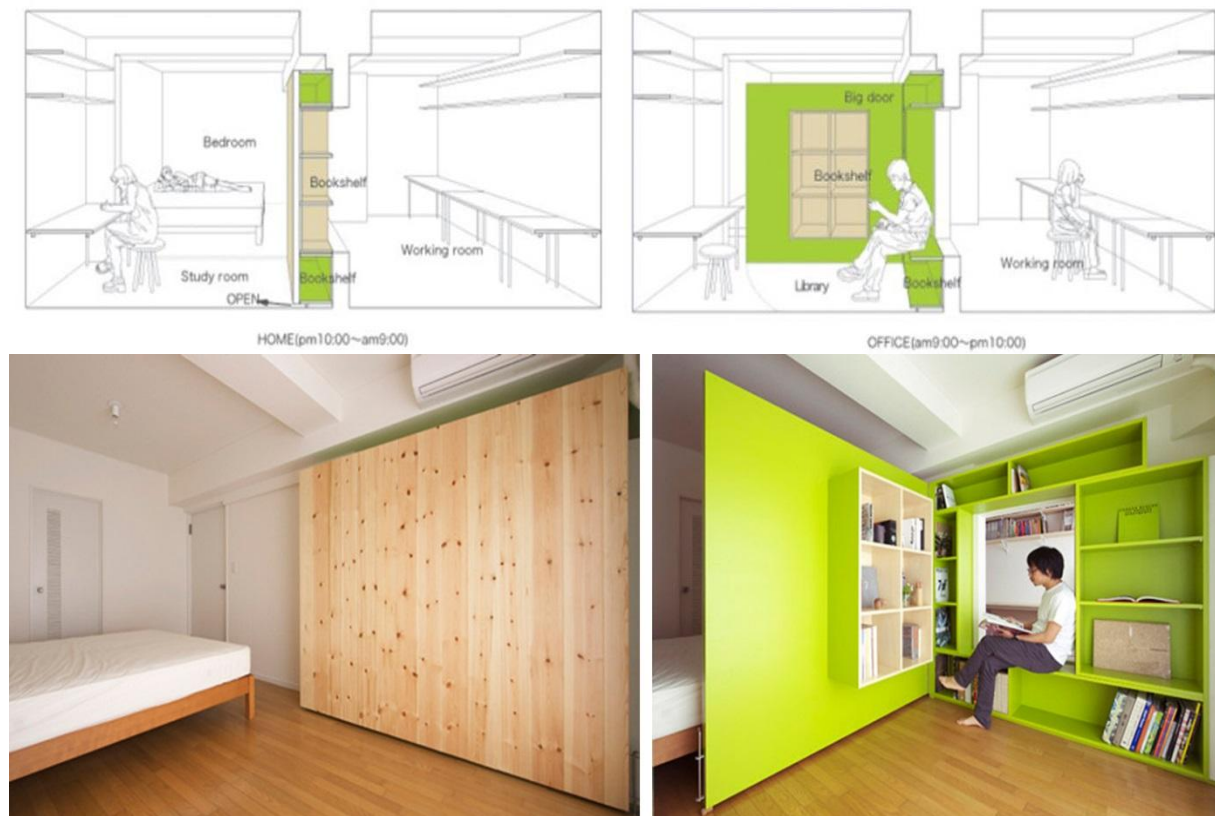
Figure.8. Example of Full Divider That Can Rotate at a Specific Angle (90 degrees) Around an Axis
