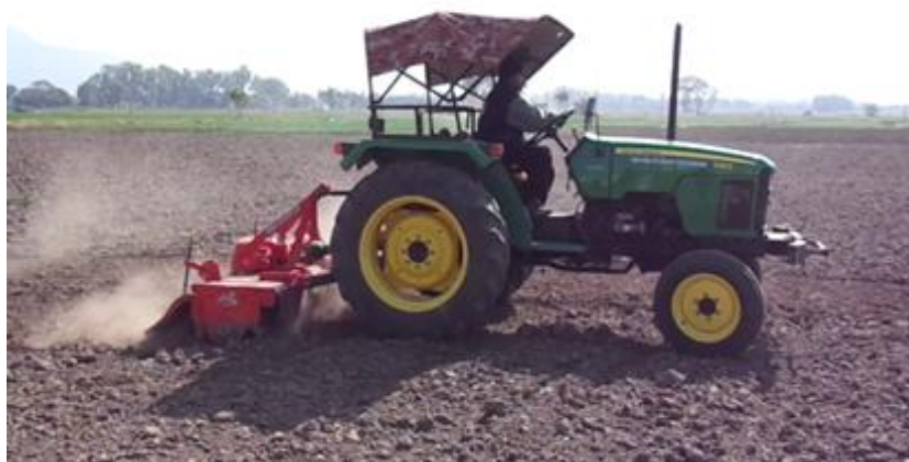
Fig. 5 Rotavator field operation with newly developed attachment
