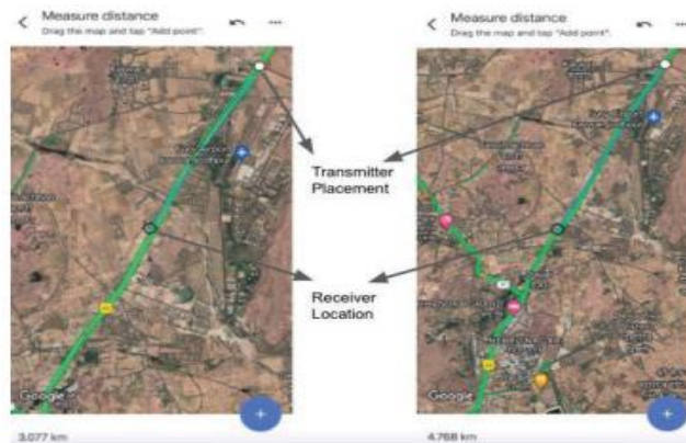
Fig. 6: Picture of the maps showing the achieved communication range for 100% data reception and 20% data reception.
