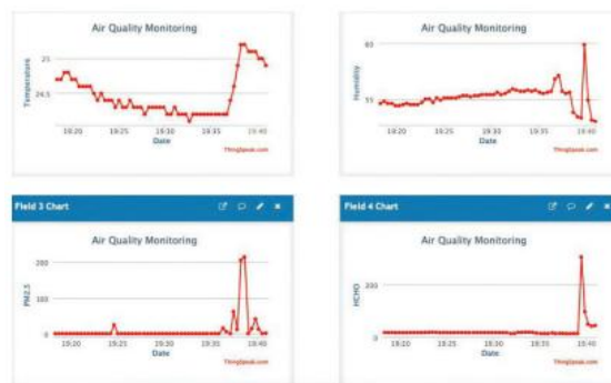
Fig. 2: Results of the implemented air quality monitoring system as seen on the ThingSpeak platform
