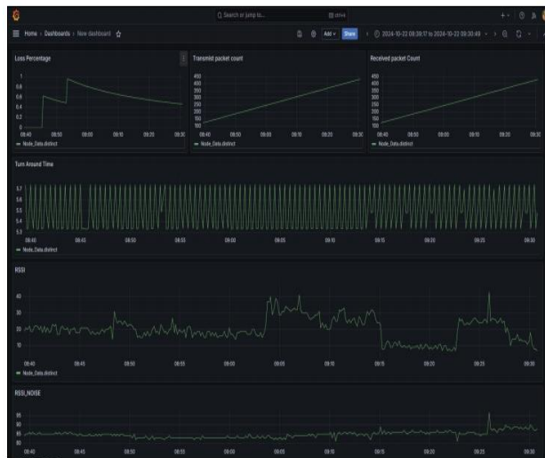
Fig. 7. Screenshot of the dashboard created to visualize the data received from all the transmitter nodes.
